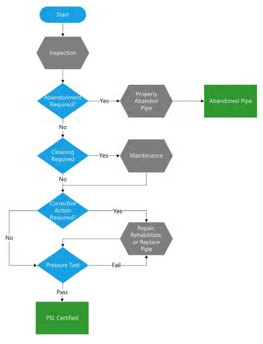
Figure 3-2 Sanitary Sewer Pipes CAWP Implementation Flowchart
