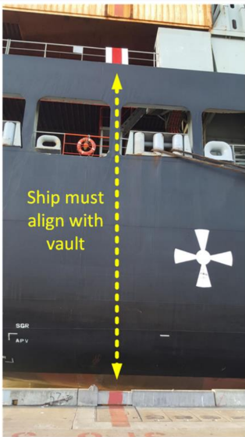
View of ship correctly aligned with marker on vault.
